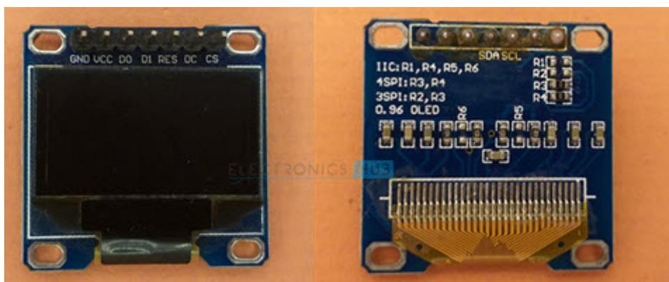
The SSD1306 OLED Driver IC has 128 x 64 bits Graphic Display Data RAM (GDDRAM). It is divided into eight pages (PAGE 0 to PAGE 7) and each page has 128 Segments. Again, each segment consists of 8-bits and each bit represents one pixel of the display.
